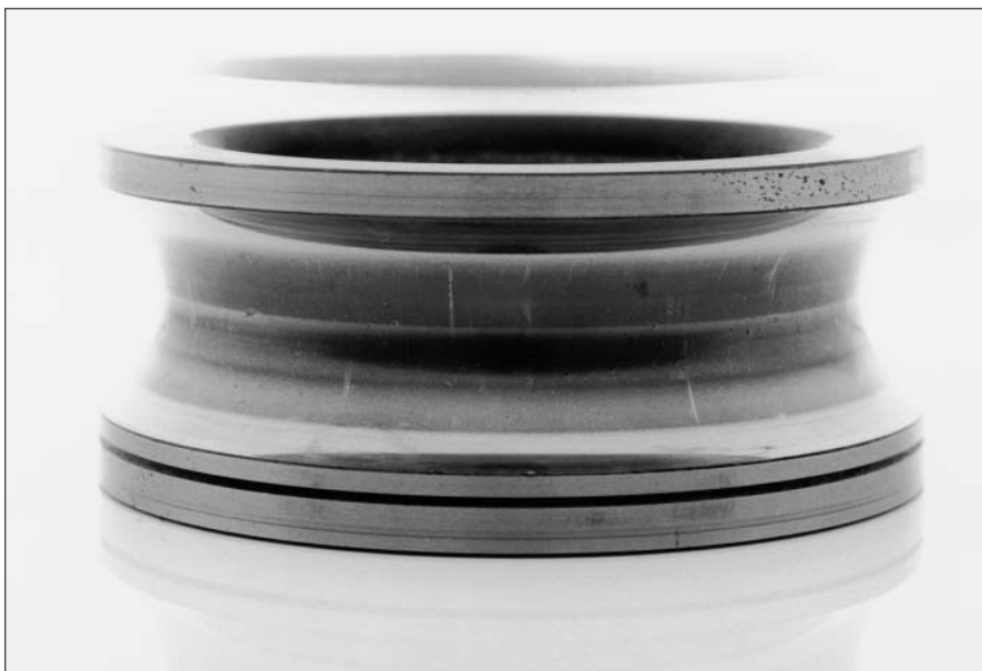
28: Track with surface wear
