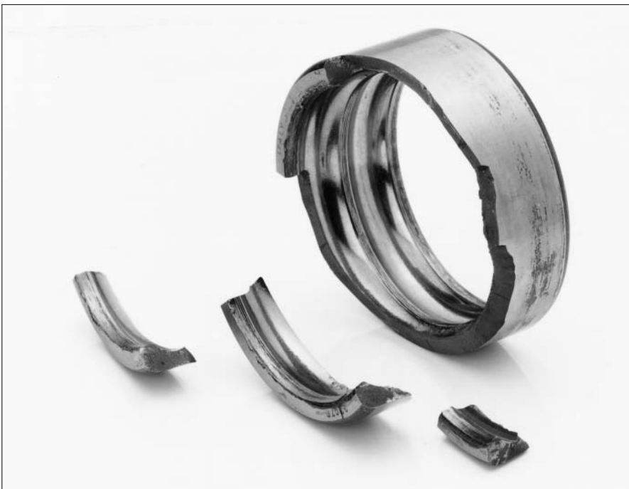
65: Crack in outer ring in circumferential direction
