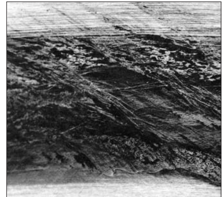
82: Seizure can arise at the roller face and lip when the lubricant supply is inadequate and loads are high.
