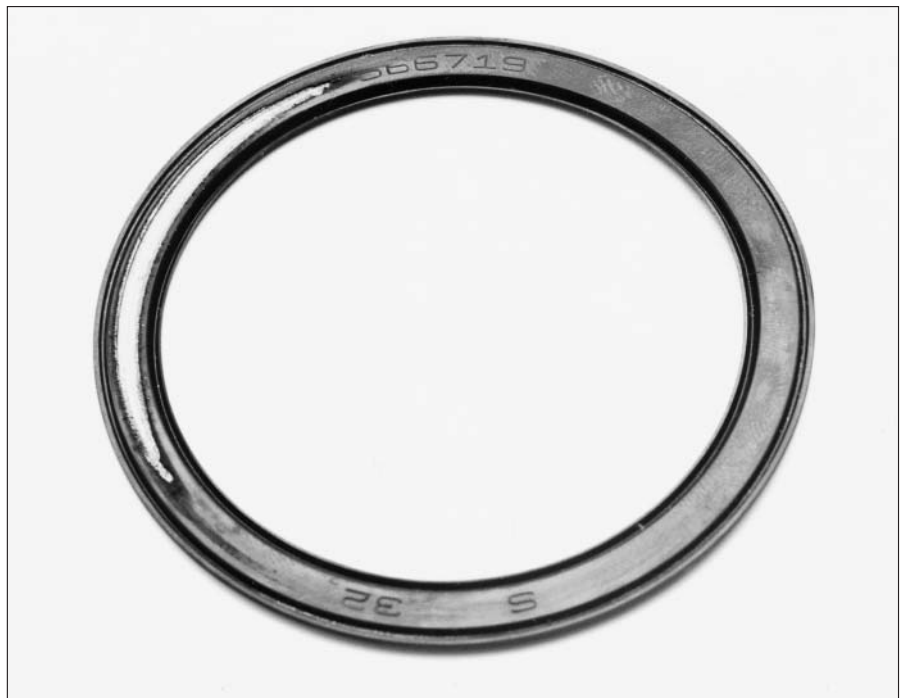
22: Seal damage due to lateral grazing
