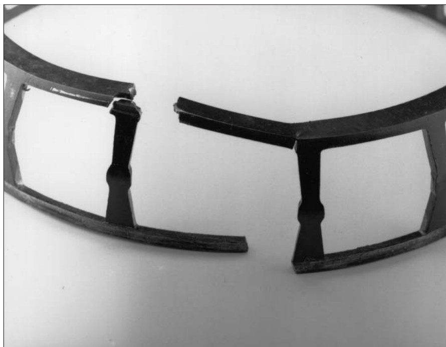
93: Disruptive fracture at the side edge of a spherical roller bearing cage
