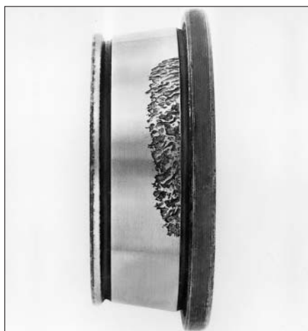
40: Tilted track on a tapered roller bearing
