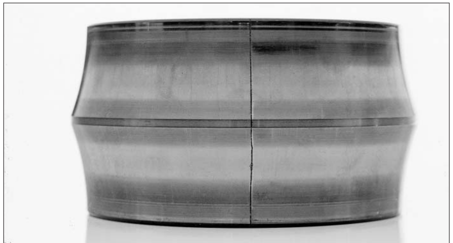
64: Axial through crack of a spherical roller bearing's inner ring
