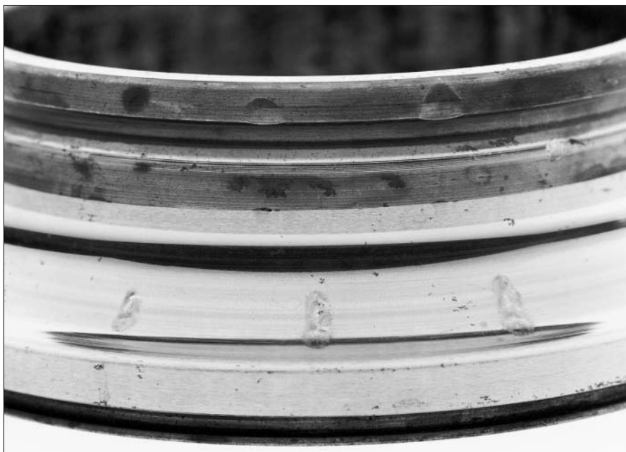
57: False brinelling on the ball bearing
