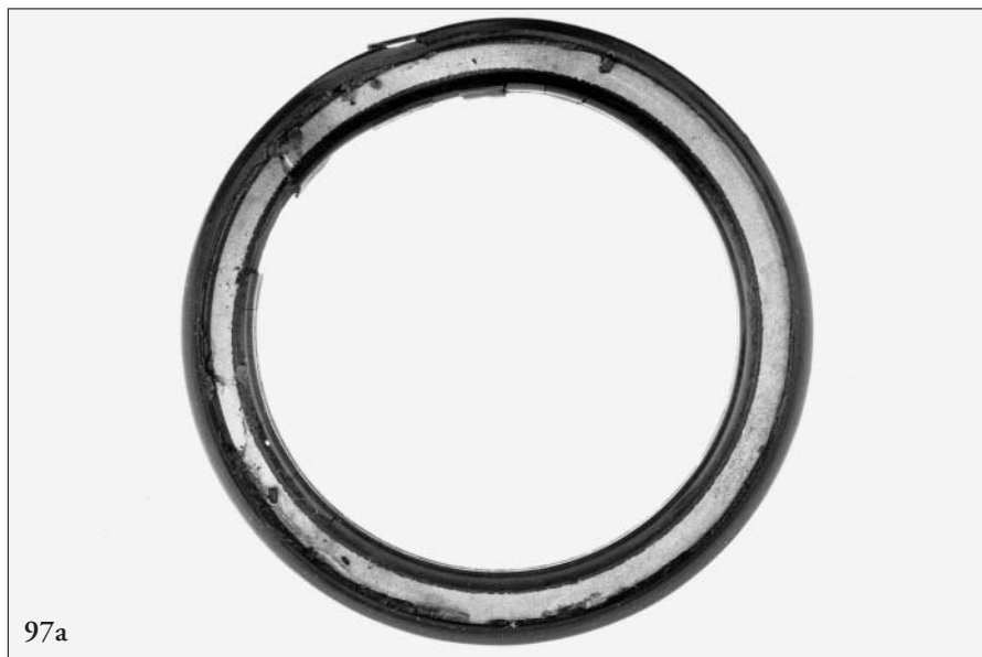
97: a: Hardened sealing with wear and fractures
