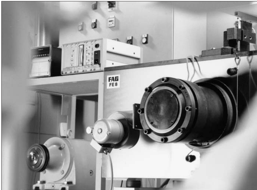
107: Test rig for determining lubricant quality
