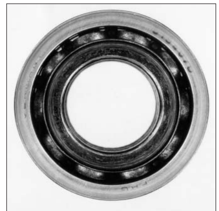
17: Circumferential scoring and cold welding at the inner ring faces as a result of inner ring creeping on the shaft
