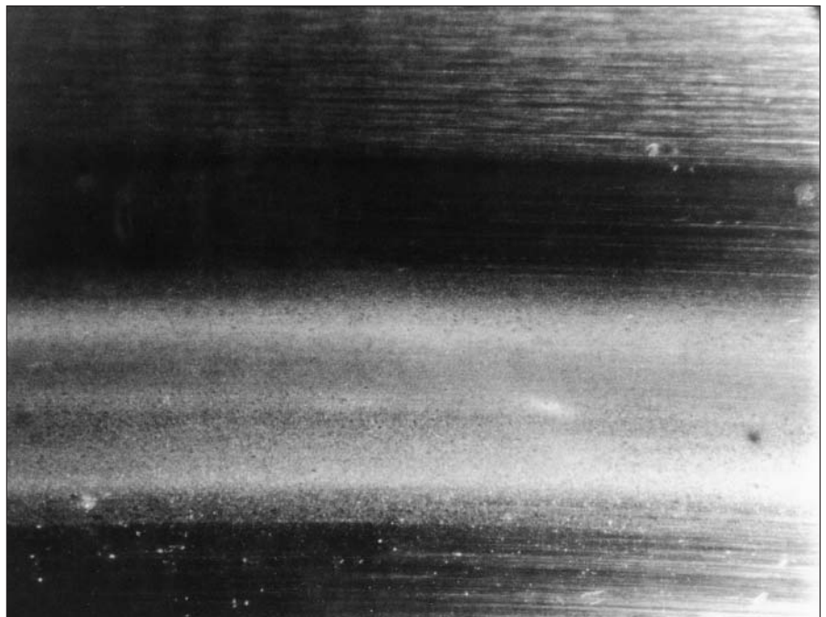
66: Worn, roughened raceway
